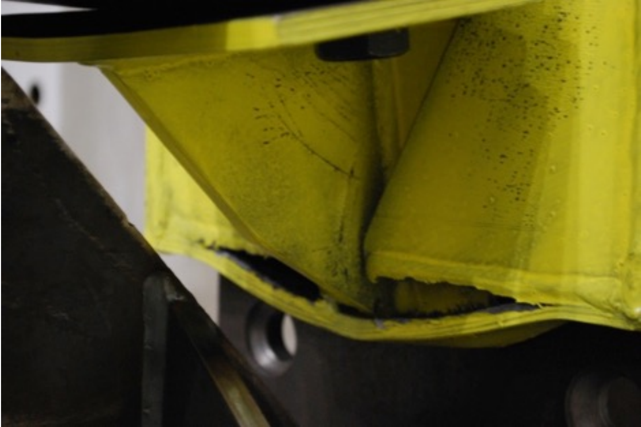
Figure 8 Condition of the Connection at the Conclusion of Testing
