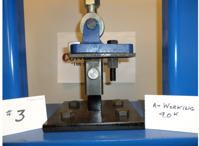
At 9.0 kips, Working Load
