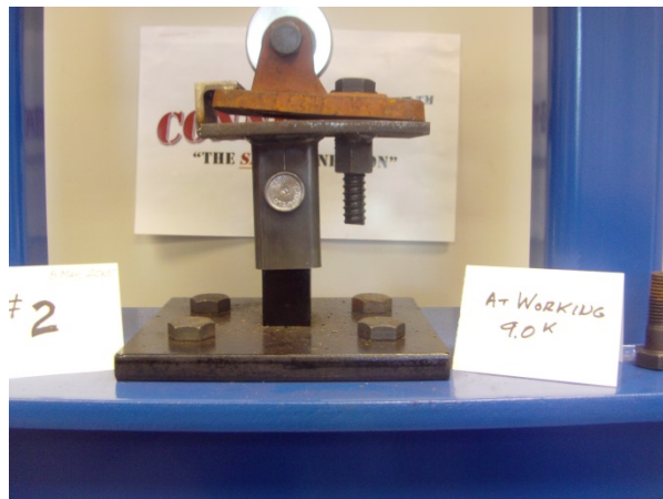
At 9.0 kips, Working Load
