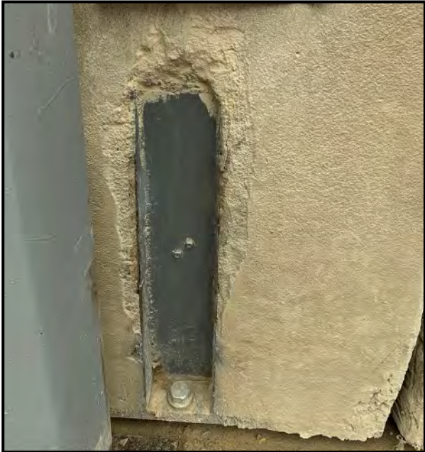
Figure 5. Crack pattern after applying 24.4 kips tension in each device
