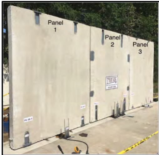
(a) Panels before bracing
